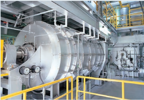
Low-temperature thermal decomposer for dioxins This machine applies heat to trapped ash in hypoxic (low oxygen) conditions, and decomposes the dioxins in the ash.
