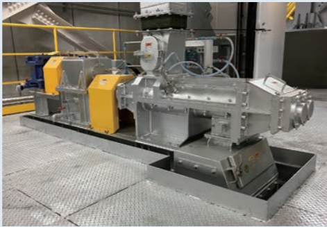
Kneader for incinerator fly ash This machine effectively treats fly ash, such as by chelation, cement solidification, and scatter prevention.
